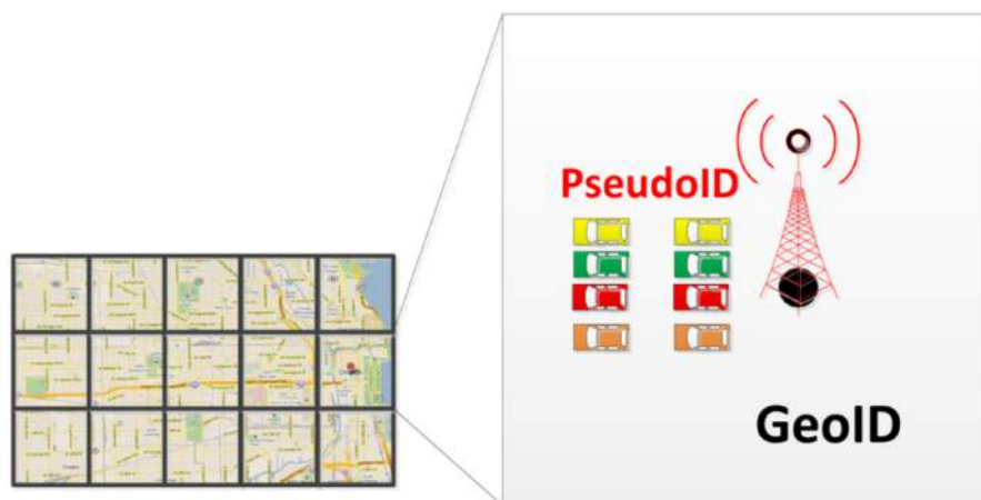
Figure 2. Each cell contains a trusted pseudonym server. GeoID is the unique identity of a cell while PseudoID is the unique identity of a vehicle inside the cell.(Yan et al., 2013; Arif et al., 2012).
